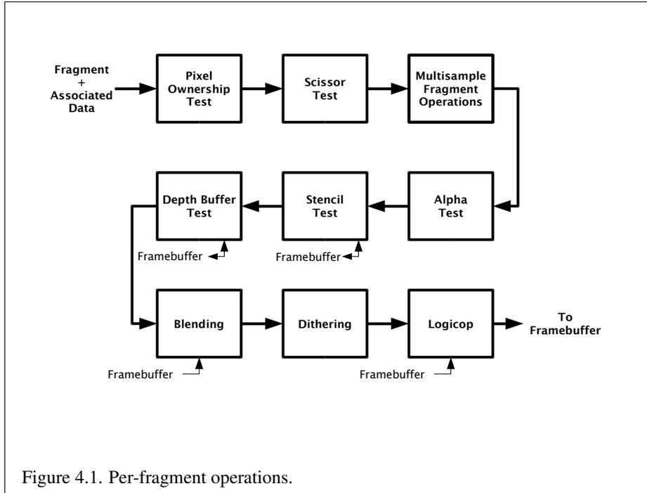
and conditions. We describe these modifications and tests, diagrammed in Figure 4.1, in the order in which they are performed.
