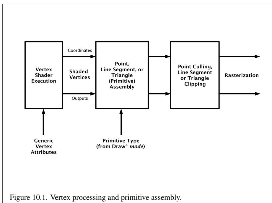
Figure 10.1. Vertex processing and primitive assembly.
