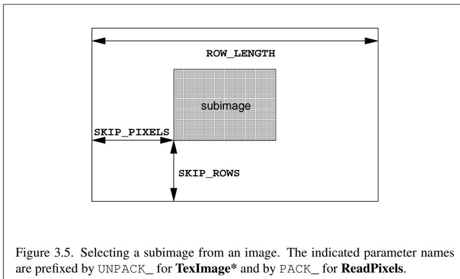
the row,  $a$  is the value of `UNPACK_ALIGNMENT`, and  $s$  is the size, in units of `GLubyte`, of an element. If the number of bits per element is not 1, 2, 4, or 8 times the number of bits in a `GLubyte`, then  $k = nl$  for all values of  $a$ .
