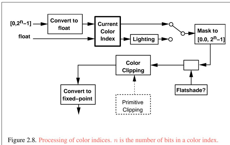
Figure 2.8. Processing of color indices.  $n$  is the number of bits in a color index.
