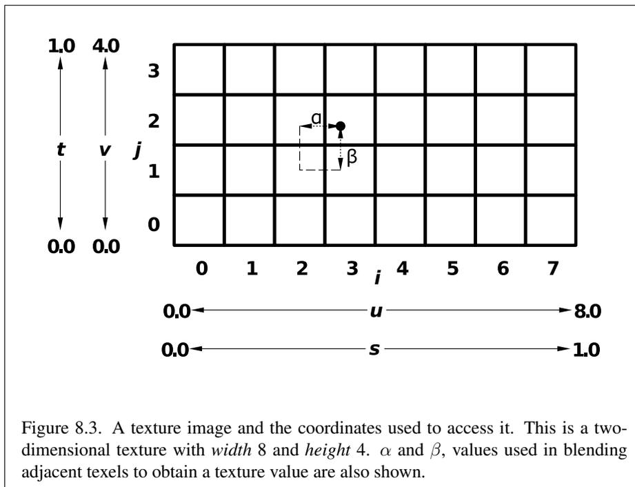
Figure 8.3. A texture image and the coordinates used to access it. This is a two-dimensional texture with *width* 8 and *height* 4.  $\alpha$  and  $\beta$ , values used in blending adjacent texels to obtain a texture value are also shown.
