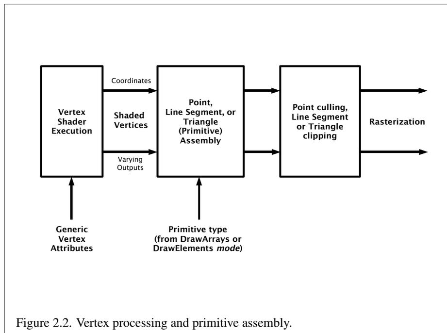
Figure 2.2. Vertex processing and primitive assembly.
