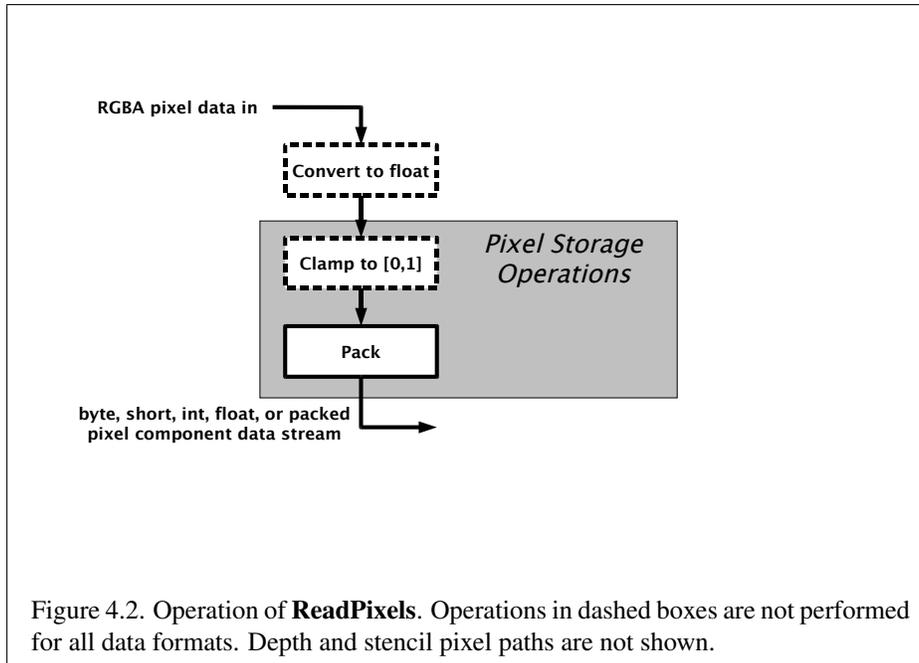
Initially, zero is bound for the `PIXEL_PACK_BUFFER`, indicating that image read and query commands such as `ReadPixels` return pixel results into client memory pointer parameters. However, if a non-zero buffer object is bound as the current pixel pack buffer, then the pointer parameter is treated as an offset into the designated buffer object.
