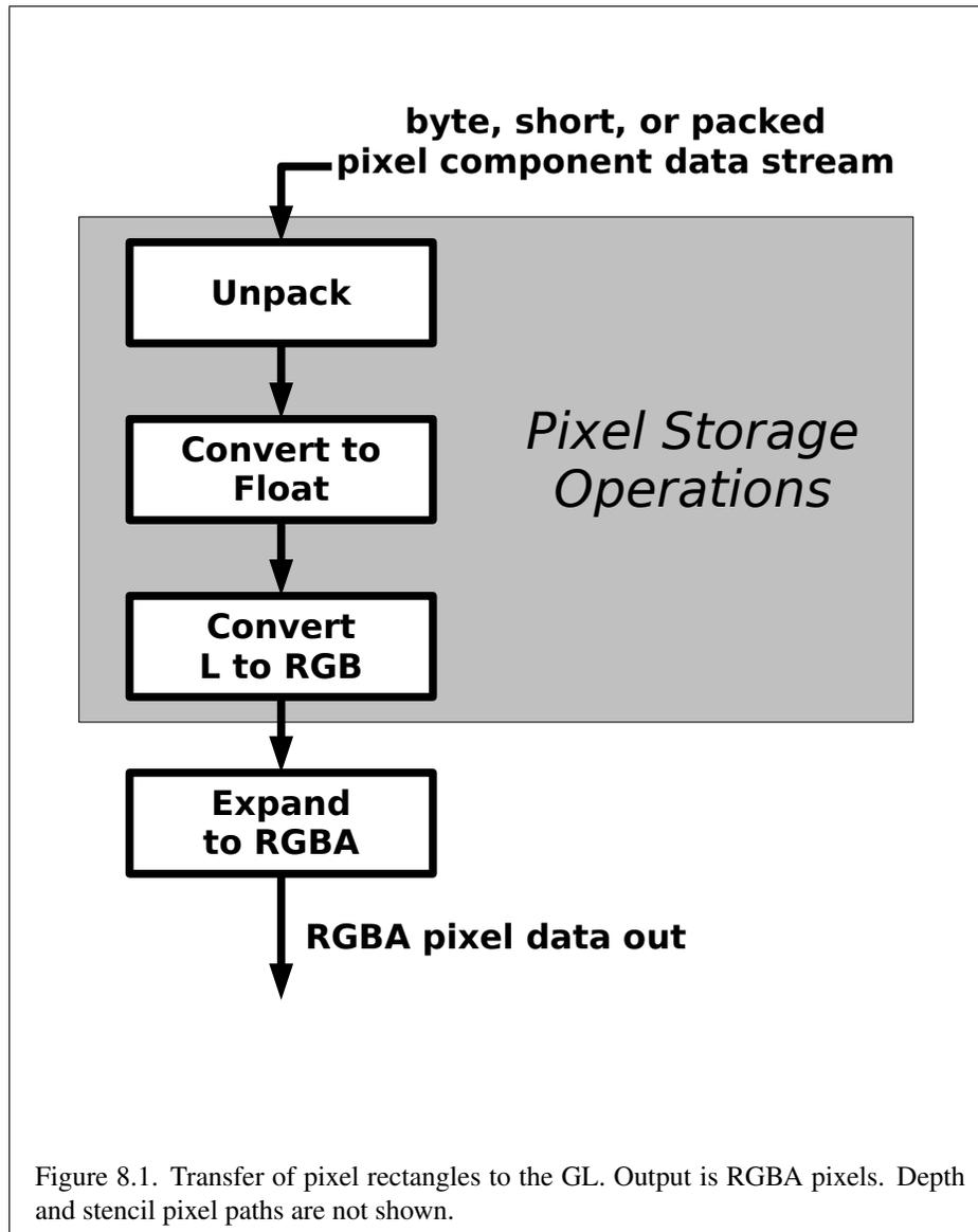
Figure 8.1. Transfer of pixel rectangles to the GL. Output is RGBA pixels. Depth and stencil pixel paths are not shown.
