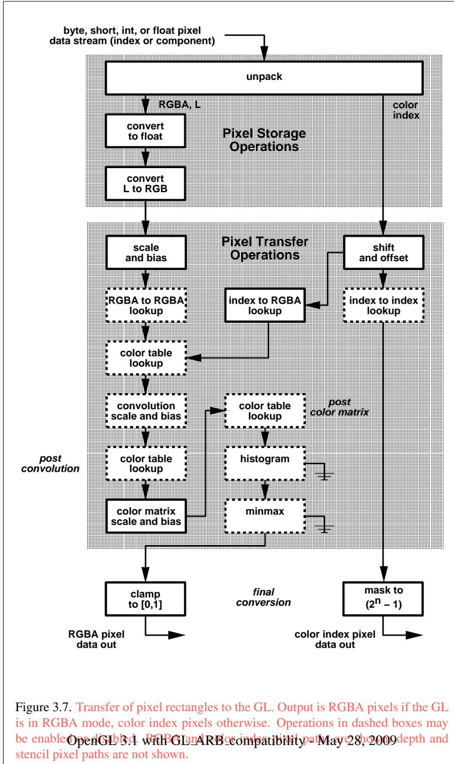
Figure 3.7. Transfer of pixel rectangles to the GL. Output is RGBA pixels if the GL is in RGBA mode, color index pixels otherwise. Operations in dashed boxes may be enabled or disabled depending on the GL implementation and capabilities. This diagram is for OpenGL 3.1 with GL\_ARB\_compatibility. May 28, 2009. Depth and stencil pixel paths are not shown.
