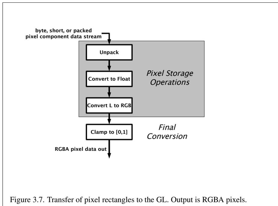
Figure 3.7. Transfer of pixel rectangles to the GL. Output is RGBA pixels.
