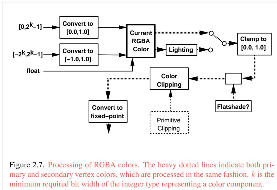
Figure 2.7. Processing of RGBA colors. The heavy dotted lines indicate both primary and secondary vertex colors, which are processed in the same fashion.  $k$  is the minimum required bit width of the integer type representing a color component.
