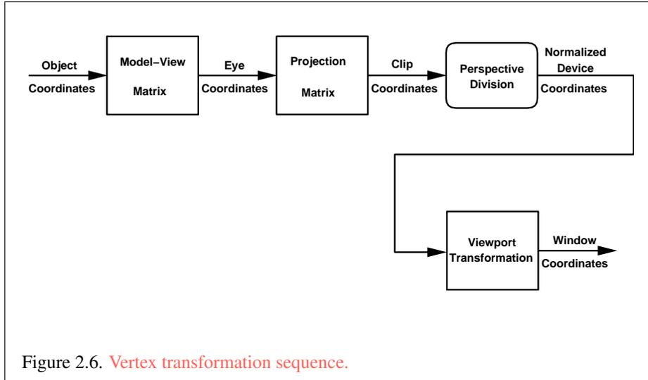
Figure 2.6 diagrams the sequence of transformations that are applied to vertices. The vertex coordinates that are presented to the GL are termed *object coordinates*. The *model-view* matrix is applied to these coordinates to yield *eye* coordinates. Then another matrix, called the *projection* matrix, is applied to eye coordinates to yield *clip* coordinates. Clip coordinates are further processed as described in section 2.15.
