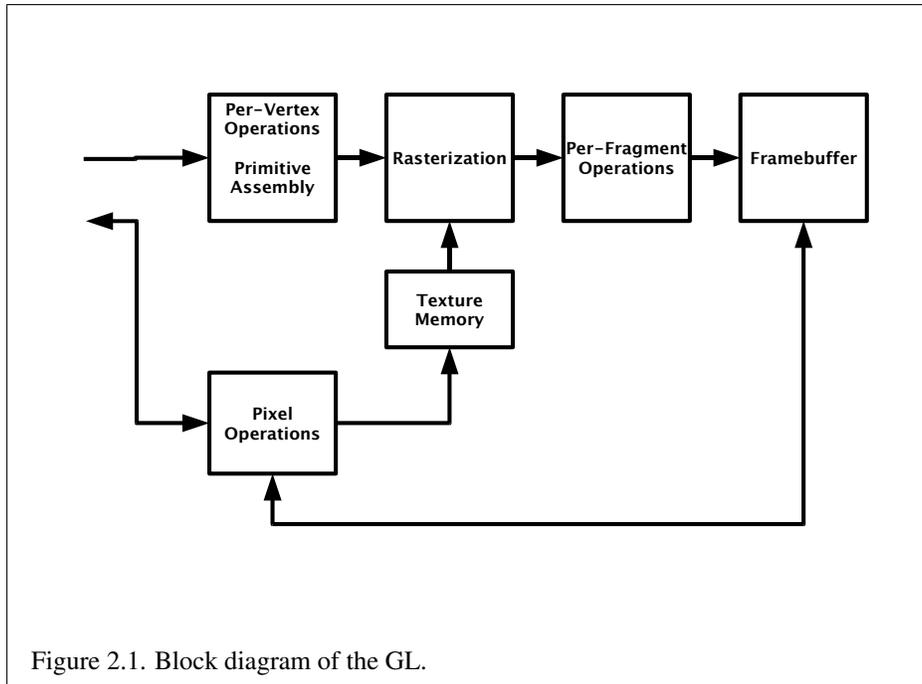
Figure 2.1. Block diagram of the GL.
