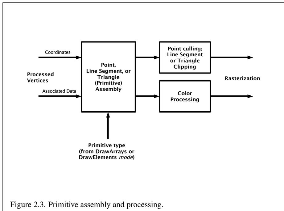
Figure 2.3. Primitive assembly and processing.
