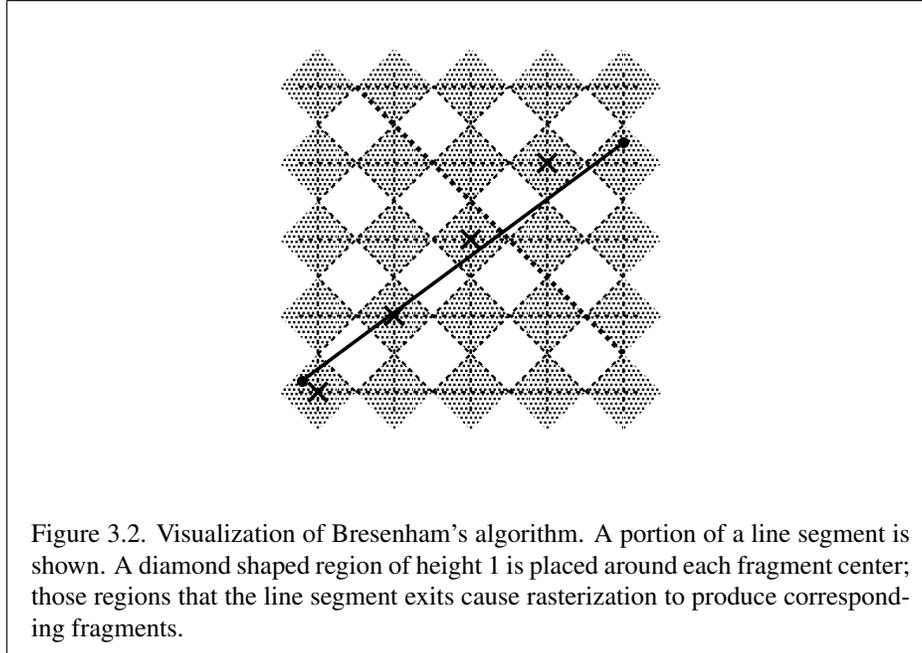
Essentially, a line segment starting at  $\mathbf{p}_a$  and ending at  $\mathbf{p}_b$  produces those fragments  $f$  for which the segment intersects  $R_f$ , except if  $\mathbf{p}_b$  is contained in  $R_f$ . See figure 3.2.
